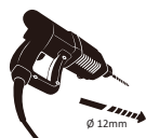
Electric drill + 12mm concrete drill bit
